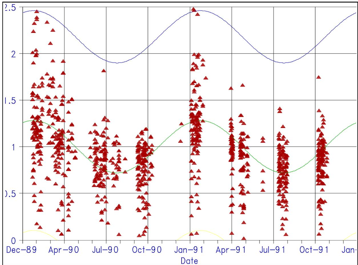
Figure 5. Seasonal variation, best-fit sinusoid, and 95% confidence interval for normalized secondary neutral impedance to ground.
