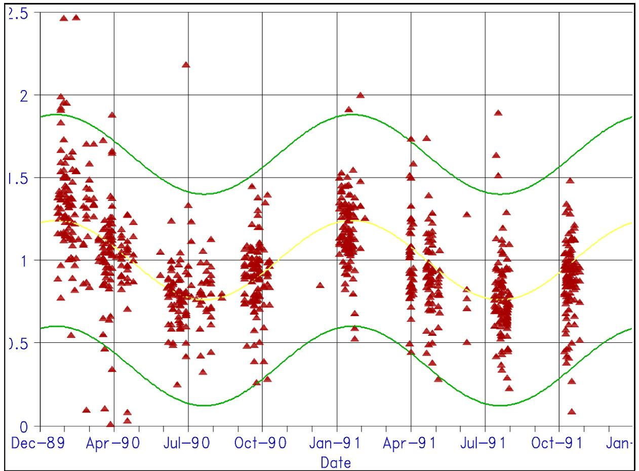
Figure 4. Seasonal variation, best-fit sinusoid, and 95% confidence interval for normalized reference ground rod impedance.
