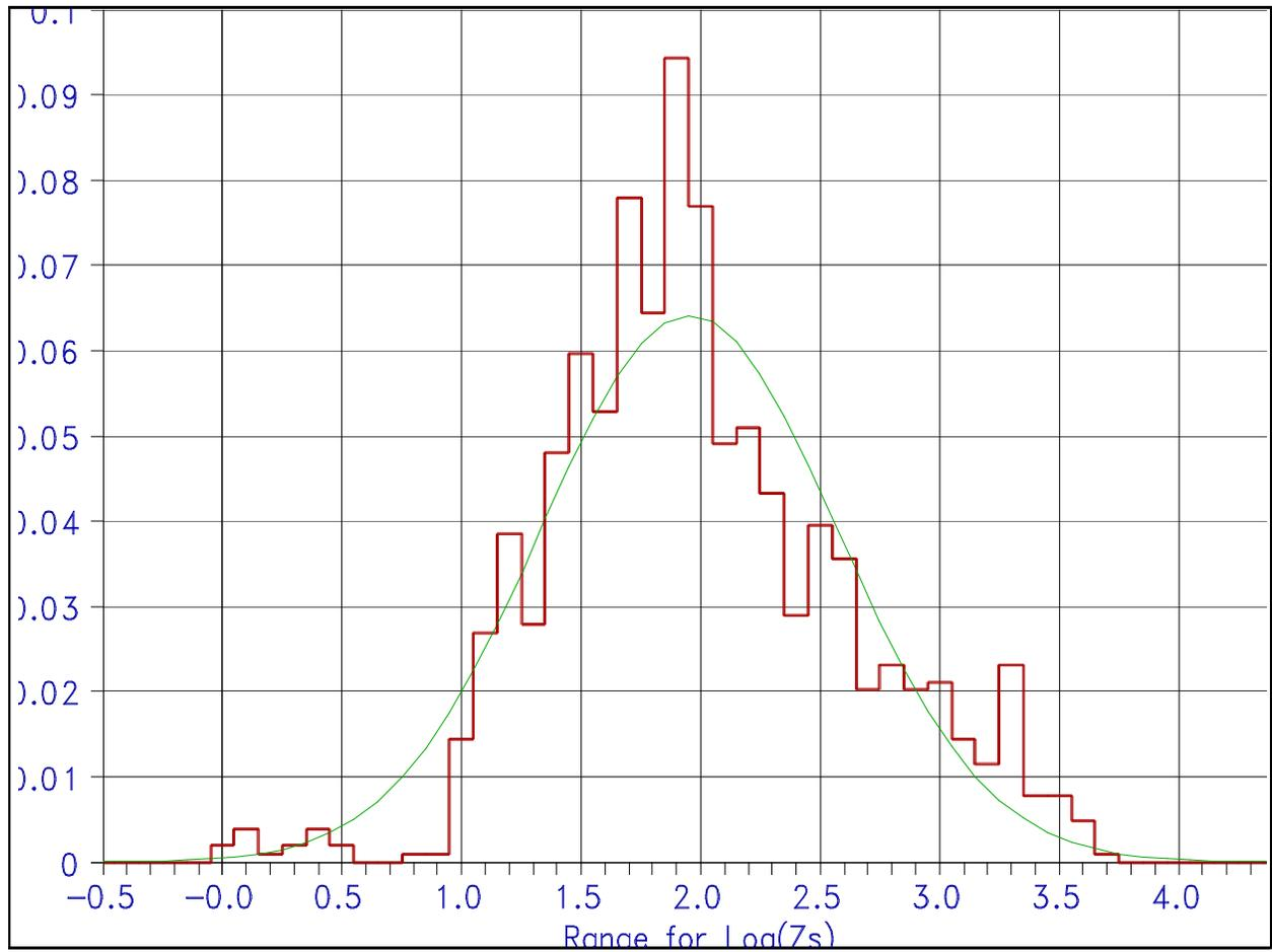
Figure 8. Frequency distribution and normalized distribution for the secondary neutral impedance to ground,  $Z_s$ .
