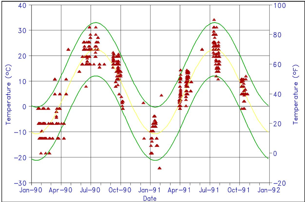
Figure 3. Seasonal variation, best-fit sinusoid, and 95% confidence interval for ambient air temperature.
