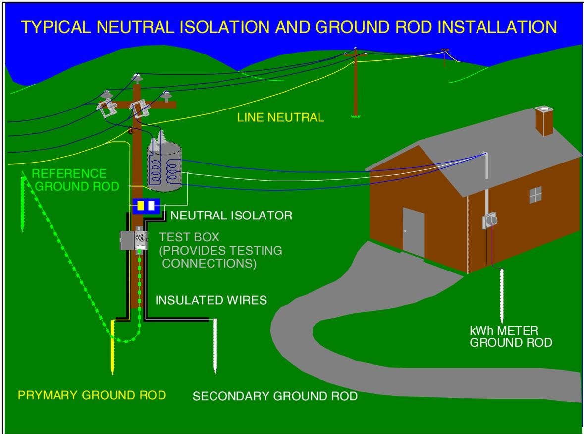
Figure 1. Typical neutral isolation and reference ground rod installation.
