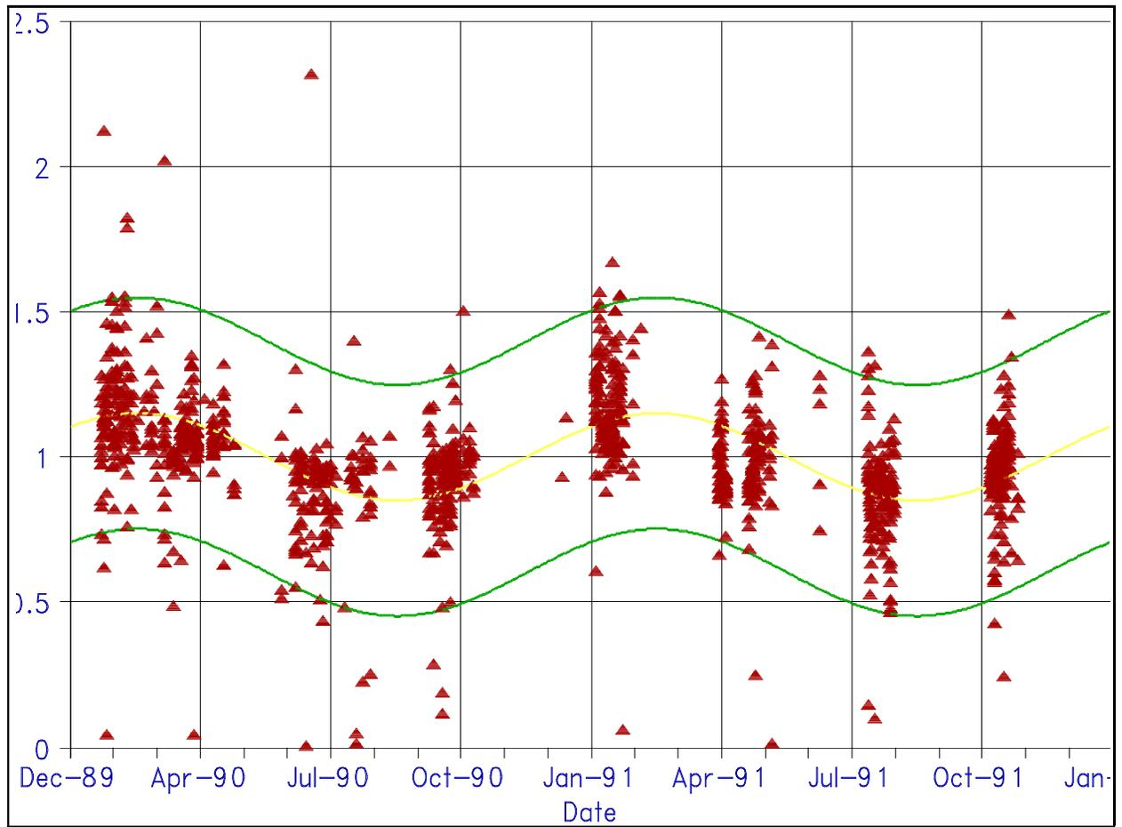
Figure 6. Seasonal variation, the best-fit sinusoid, and 95% confidence interval for normalized primary neutral voltage.
