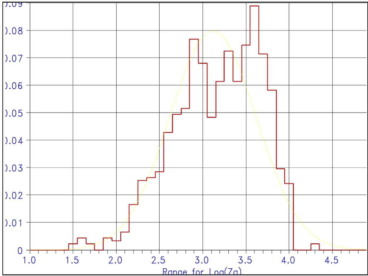
Figure 7. Frequency distribution and normalized distribution for the reference ground rod impedance to ground,  $Z_g$ .
