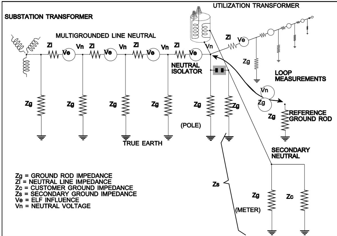
Figure 2. Grounding circuit formed by the neutral wire.
