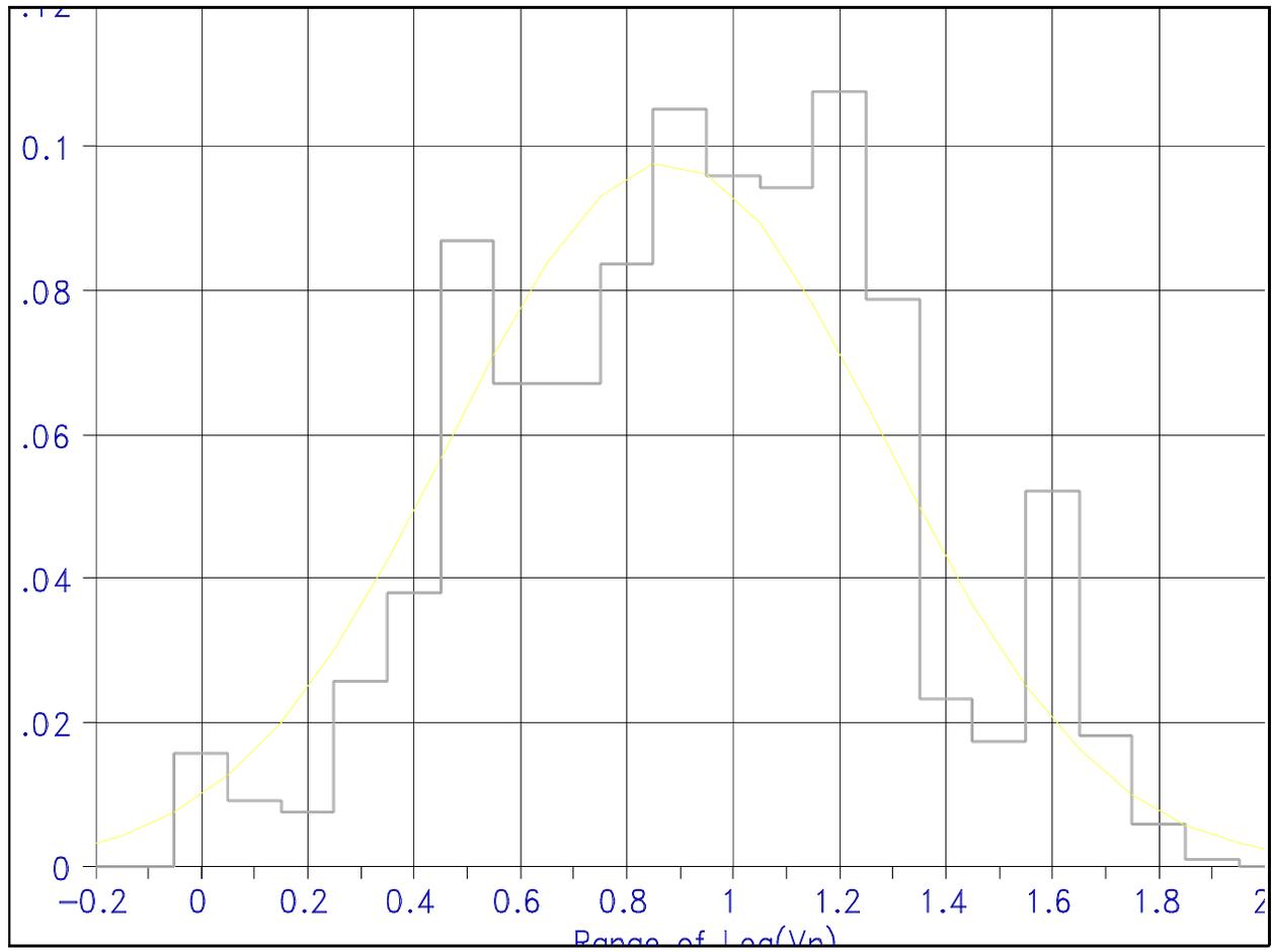
Figure 9. Frequency distribution and normalized distribution for the 76 Hz neutral voltage  $V_n$ .
